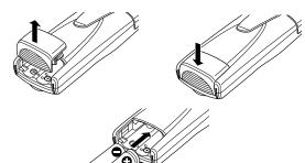
**IMPORTANT** — The batteries supplied with this product are rechargeable Ni-MH, 1300mAh. When replacing batteries, never use other types of batteries or conventional alkaline batteries.
